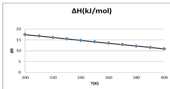
Figure 1. Diagram of the enthalpy changes for the synthesis material 1- (4-nitrophenyl) -1 hydrogen Tetrazole at different temperatures.
