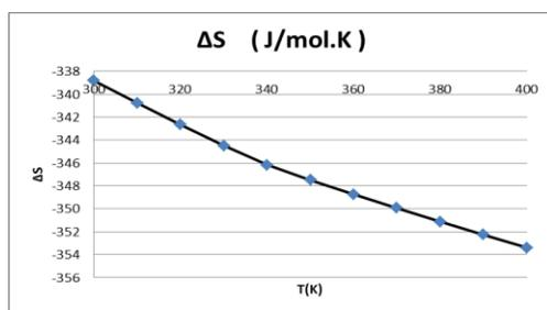
Figure 2. Diagram of the entropy changes for the synthesis material 1- (4-nitrophenyl) -1 hydrogen Tetrazole at different temperatures.
